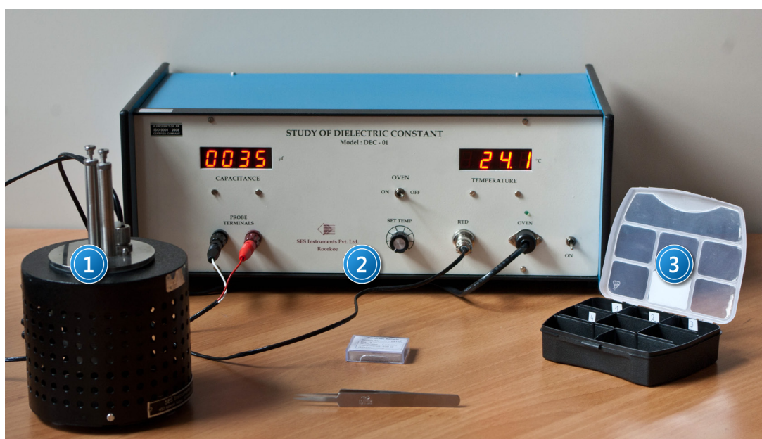
Picture 1. Setup for measuring the dielectric constant of ferroelectric materials: 1 – heating oven with capacitor; 2 – RLC bridge; 3 – set of samples (ferroelectric crystals).
